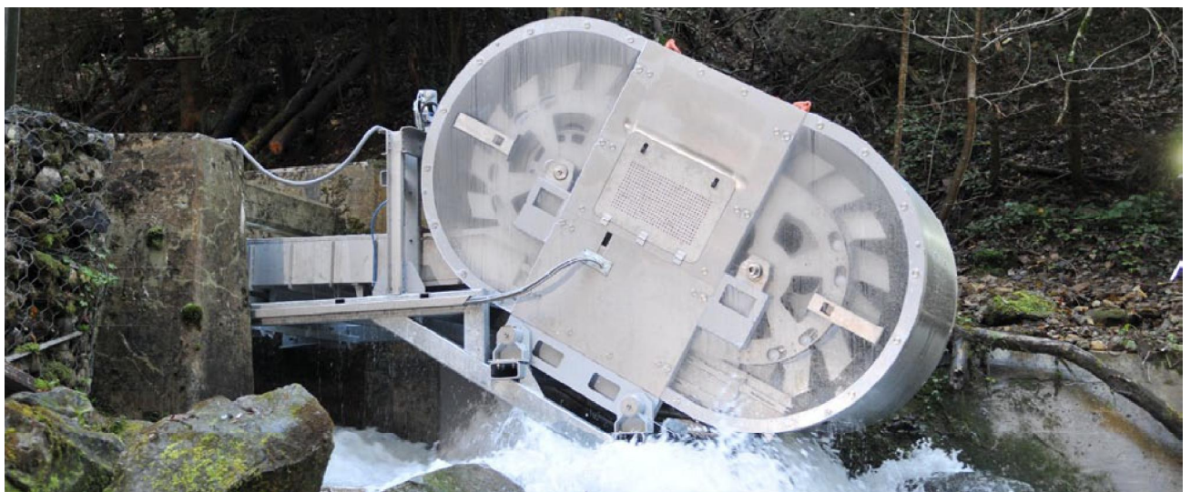
The Steffturbine is positioned above the water
