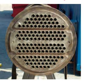
Tubular Heat Exchangers are vital to the operation of a plant. Failures are considered unacceptable both economically and environmentally. Failure is usually caused by corrosion or erosion of the tube wall. Regular inspection is the best means of detecting wall loss at an early stage.
