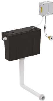
Sensorflow 21 single flush 6 litre cistern, side inlet, panel mounted touch free sensor actuation, adjustable to low water volumes (4.5 or 4 litres), internal overflow, flushpipe included
