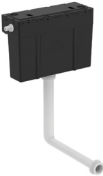
Dual flush 6/4 adjustable to 4/2.6 litres flush cistern, side inlet, pneumatic actuation with internal overflow & flushpipe included
