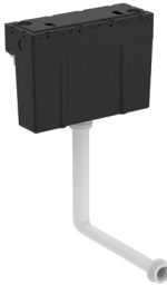
Dual flush 6/4 adjustable to 4/2.6 litres flush cistern, top/bottom inlet, pneumatic actuation with internal overflow & flushpipe included
