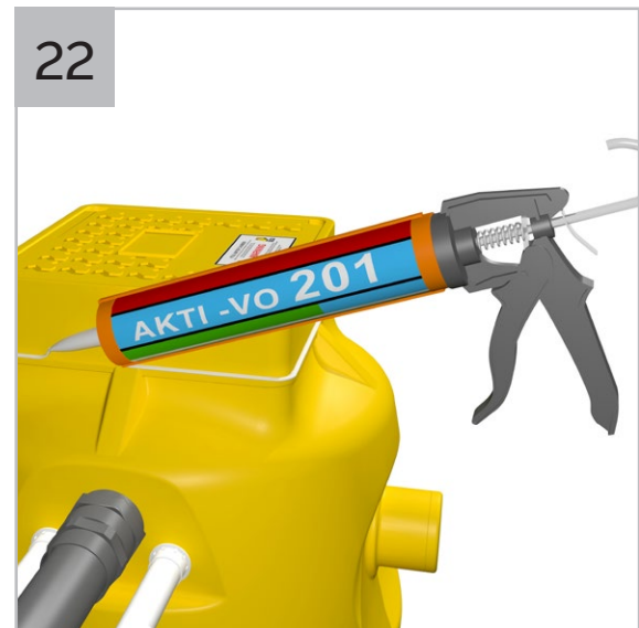
22 Once chamber has been filled with water, apply Delta AKTI-VO 201 (swellable mastic) to the entire external lip locator of Chamber.
