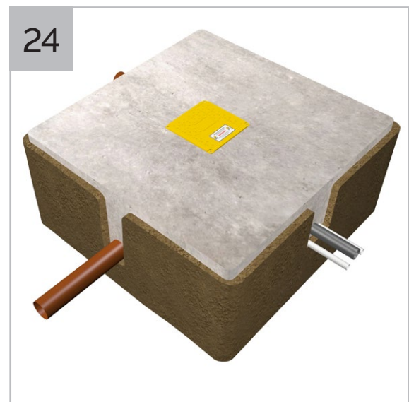
24 Allow concrete to cure.
